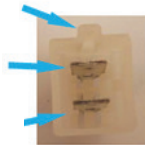
front view plug-in housing with flat plug-in tongue
