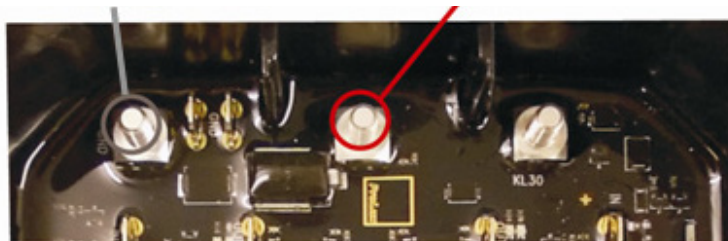
Terminal power supply +12 V / +24 V
